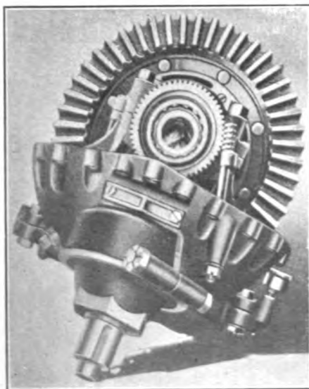
Fig. 2—Differential and bevel drive unit which are separately assembled
